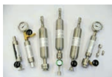
Gas Leak Standards
